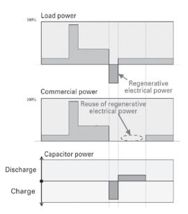
Fig. 8: Power pattern when regenerative electric power is generated
